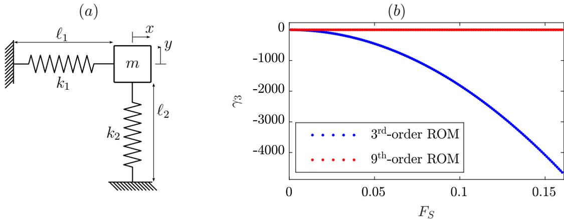
Figure 1: A schematic diagram of the simple oscillator, used to motivate this work, is shown in panel (a). The value of the ROM parameter,  $\gamma_3$ , as the force scale factor,  $F_S$ , is varied is shown in panel (b).
