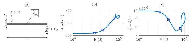
Figure 1: (a) Schematic diagram of beam+cubic spring (b) Main branch of dNNM1 (c) Damping ratio with respect to energy. Squares: Solution points where a PGD mode is added.
